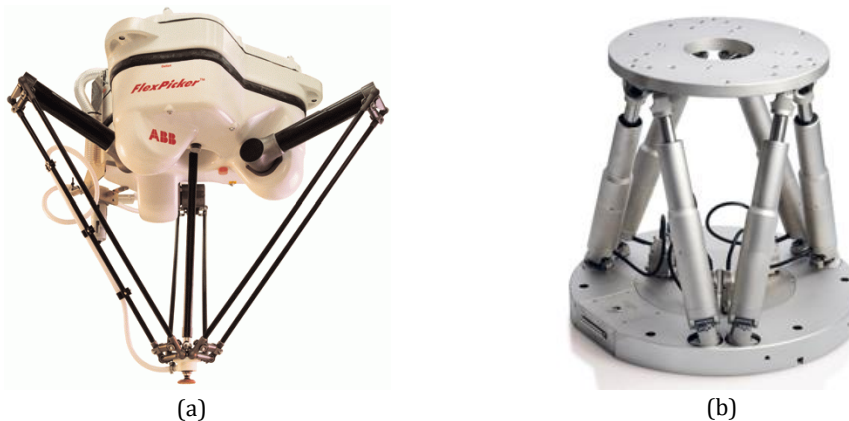
Figure 1: A delta robot (a); a Gough-Stewart platform (b).
