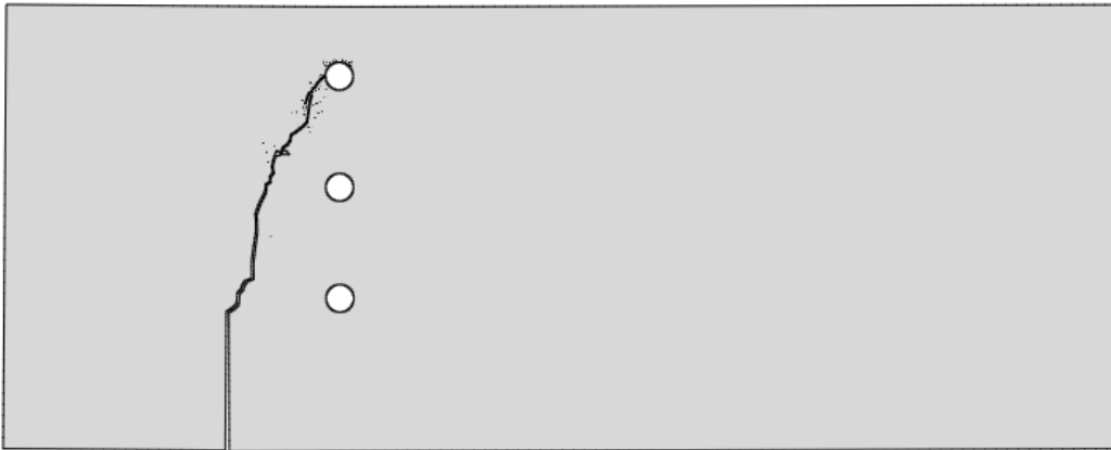
Fig. 14: Selectively Activated CZM; G_{crit} = 0.175 N/mm (1 lbf/in). Scale factor=1.
